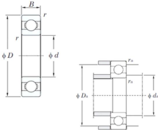
6301 Bearing 2D drawings and 3D CAD models
